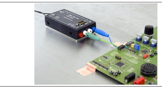
Figure 2: Opto-Box 100 in LIN mode, measurement set-up for measurement during development
