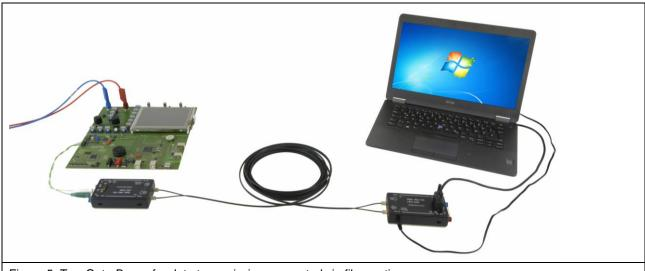
Figure 5: Two Opto-Boxes for data transmission connected via fiber optics
