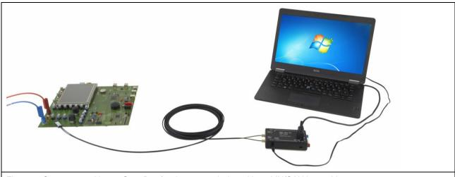
Figure 7: One sensor with one Opto-Box for data transmission without LIN/CAN bus cable
