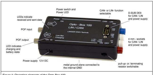
Figure 1: Operating elements of the Opto-Box 100
